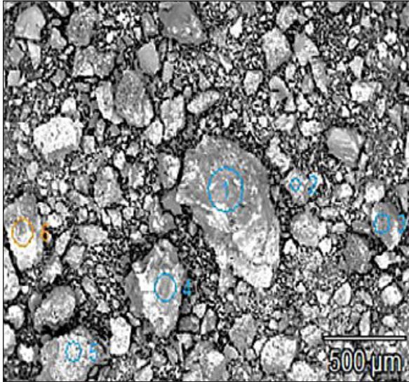
Figure 5. SEM image of geopolymer obtained from galvanic sewage sludge
