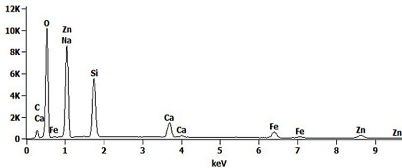
Figure 7. EDS analysis (research area – 2) of geopolymer obtained from galvanic sewage sludge
