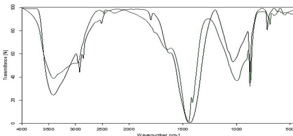
**Figure 9.** FTIR spectra of galvanic sewage sludge (black) and geopolymer obtained from galvanic sewage sludge (green)
