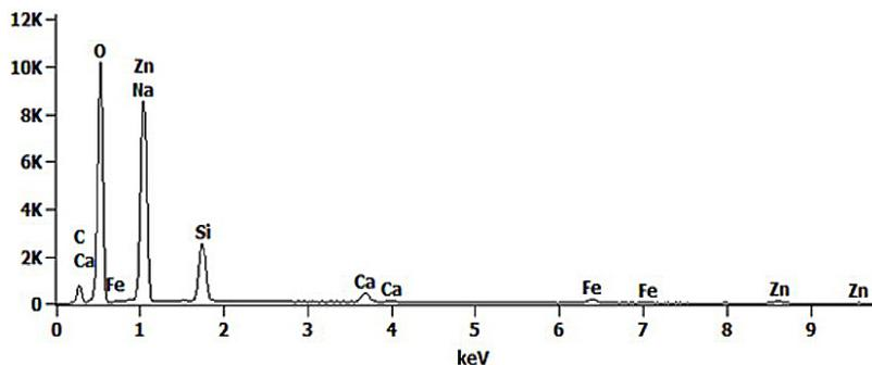
Figure 8. EDS analysis (research area – 3) of geopolymer obtained from galvanic sewage sludge
