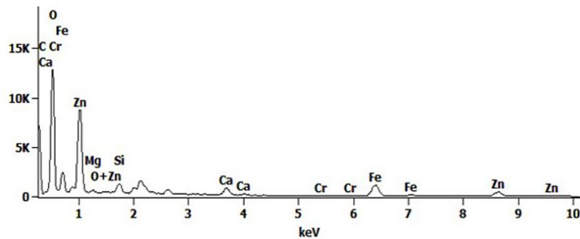
Figure 2. EDS analysis (research area – 1) of galvanic sewage sludge
