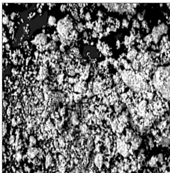
**Figure 1.** SEM image of galvanic sewage sludge
