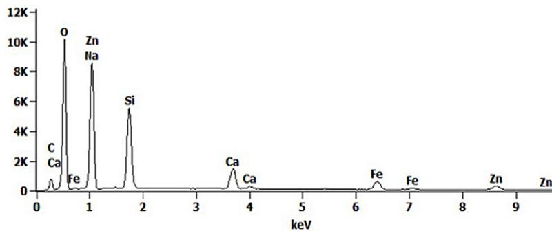
Figure 6. EDS analysis (research area – 1) of geopolymer obtained from galvanic sewage sludge
