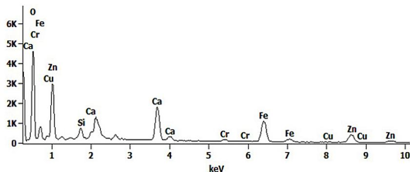
Figure 4. EDS analysis (research area – 3) of galvanic sewage sludge
