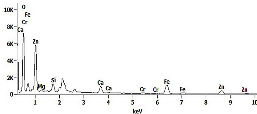
Figure 3. EDS analysis (research area – 2) of galvanic sewage sludge
